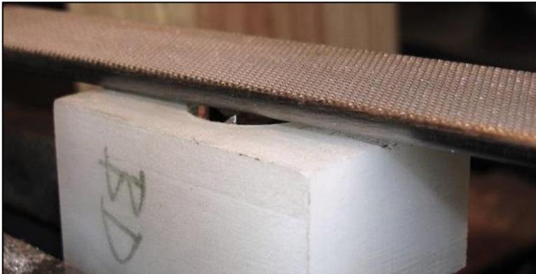
File all teeth down level with the surface of the block (use the fine side of the file).
