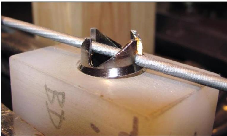
Using a 1/8" round file cut down the root of the tooth (bottom of the "V" between the teeth).
