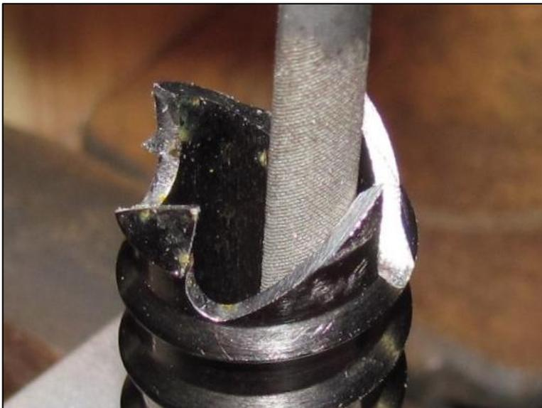
Using the round side of the file remove any burrs along the inner edge of the tooth.
