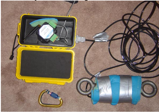
Figure 3: Typical S-type load cell attached with quick disconnect to wireless v-link data logging system.
