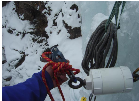
Figure 5(left) weighing the test mass, & 6 (right) displaying the results of why a stopper knot is necessary – note the over camming of the Grigri that allowed no slip.
