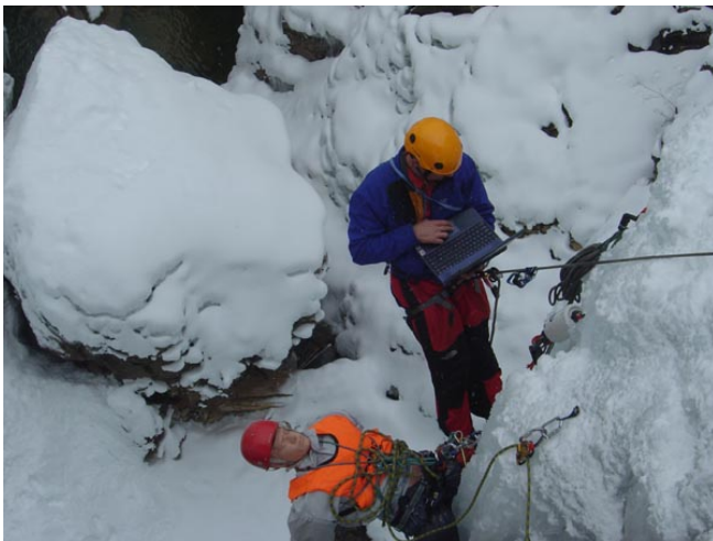
Figure 2: Configuring the data collection node and preparing the test weight on the “Rhythm Method” WI5 in Ouray, Colorado.
